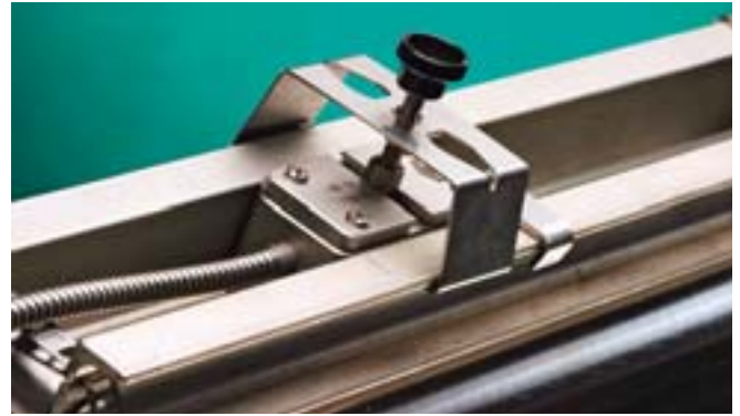
Clamp-on sensor does not get in contact with the medium
